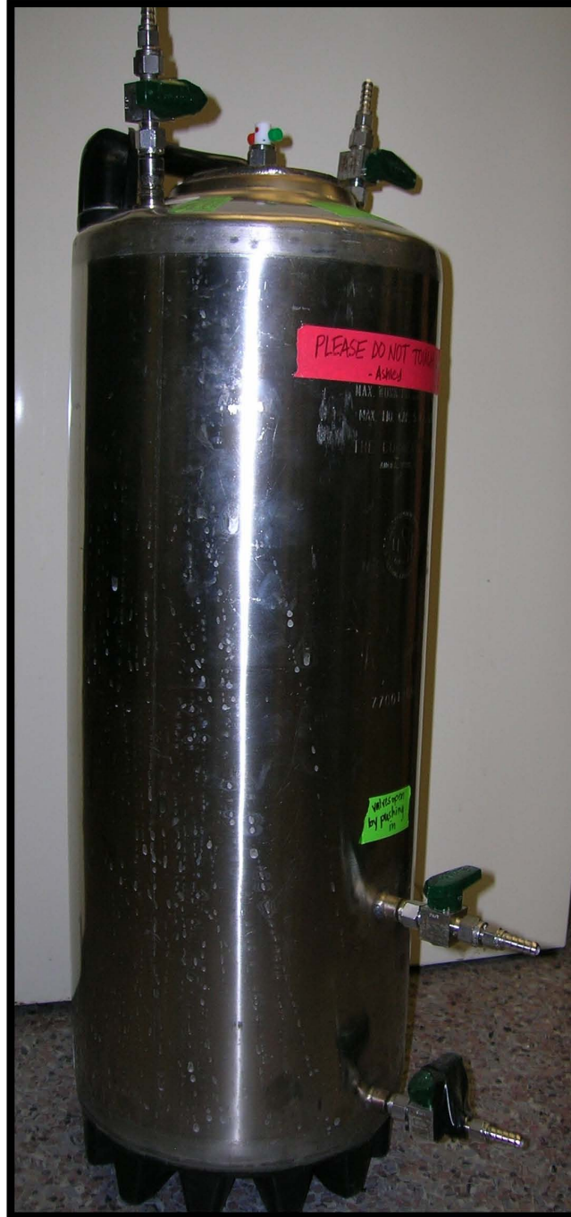
Figure C.1 Photo of canister #1 modified with valves and Mininert® sampling port.
