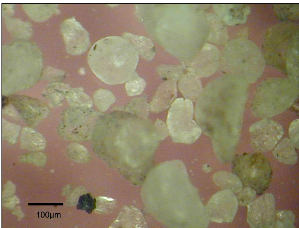
Figure 3-28. Microphotograph of round, clear particles collected after live firing of a 155-mm howitzer with M1 single-base propellant at Fort Lewis firing point 3409.
