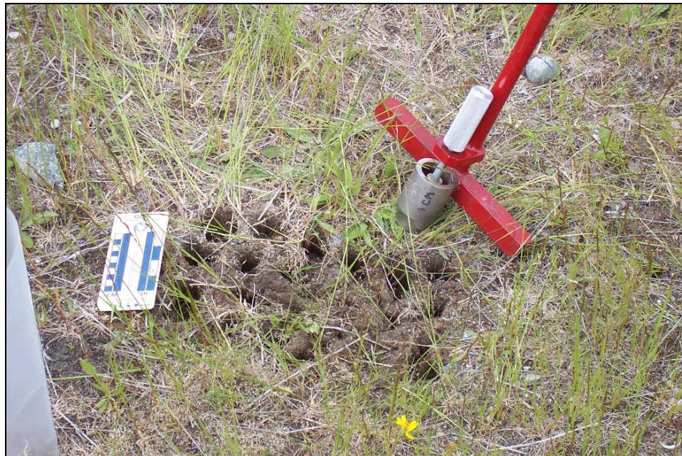
Figure 3-12. Layout of contiguous sampling at range 59, Fort Lewis, Washington, for simulating a single discrete sample with six 4-cm-diameter cores. Quadruplicate samples were collected from the center of the 20-m x 10-m decision unit positioned 5–15 m behind the firing line.
