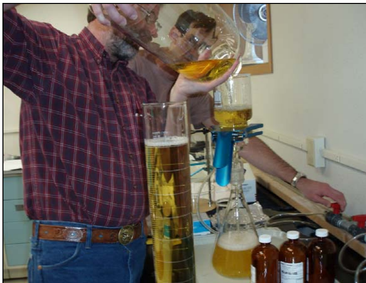
Figure 2-13. Filtering propellant burn area sample (M205-a).
