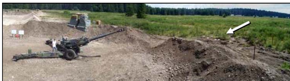
Figure 3-13. Fort Lewis firing point 3409, at location of 155-mm howitzer, in front of which live-fire residues and soil samples were collected. Arrow marks sampled area beyond the gravel berm.
