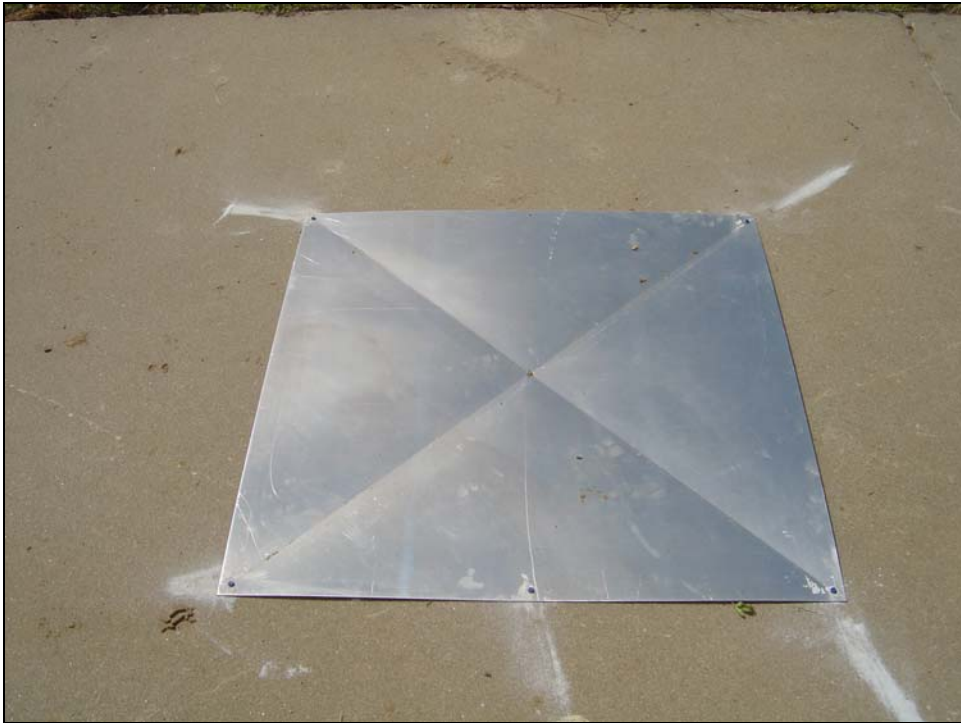
Figure 6-4. Aluminum witness plate.
