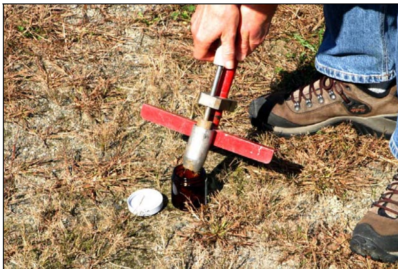
Figure 3-1. Coring tool designed at CRREL for multi-increment sample collection.
