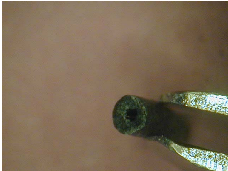
b. Single-perforated propellant grain used to fire the 155-mm howitzer projectiles.
