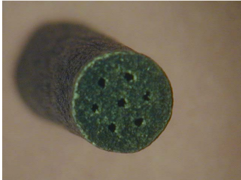
a. Seven-perforation propellant grain used to fire the 105-mm howitzer projectiles.
