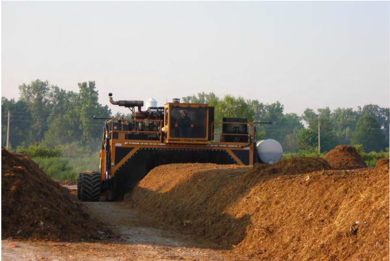
**Figure A-1. Windrow being turned by a windrow turner at PBOW.**
