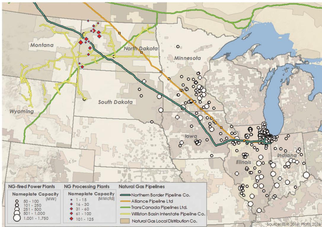
**Fig. 11.** (Color) Natural gas system in North Dakota and related electric power infrastructure (map data from ESRI 2016; Platts 2016 Q1)
