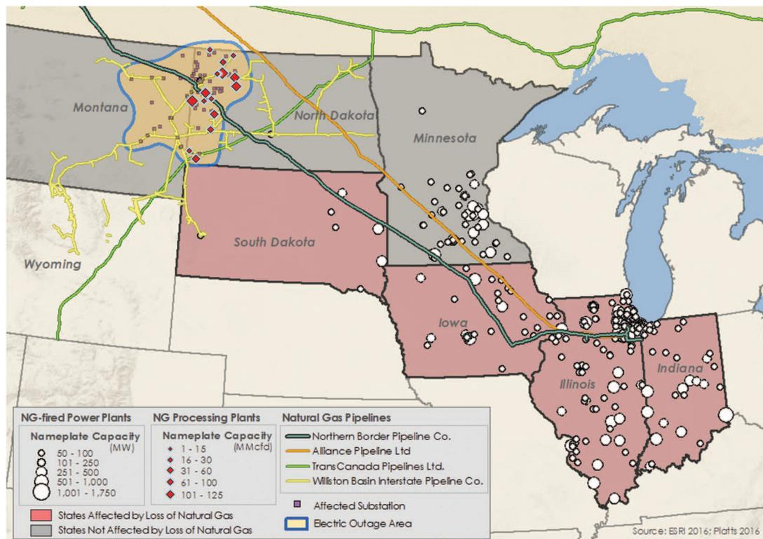
Fig. 12. (Color) Simulation results for the North Dakota case study (map data from ESRI 2016; Platts 2016 Q1)
