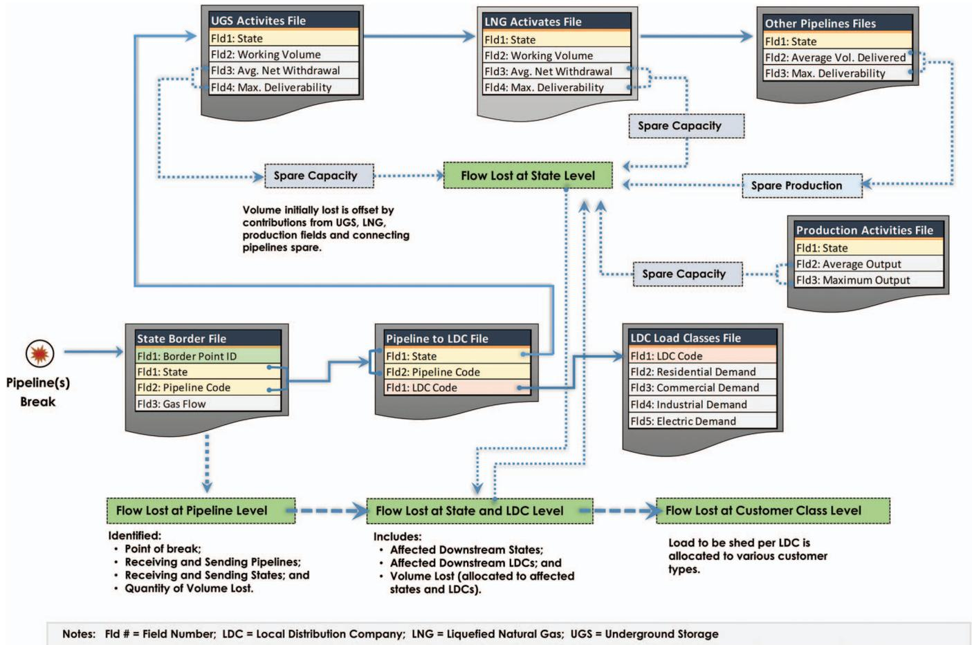
**Fig. 5.** (Color) *NGfast* relational data supporting disruption propagation approach
