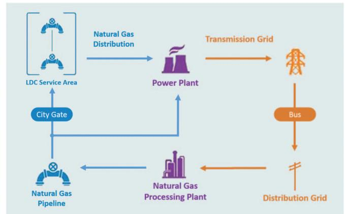
Fig. 8. (Color) Example of interdependencies between the electric power and natural gas infrastructure
