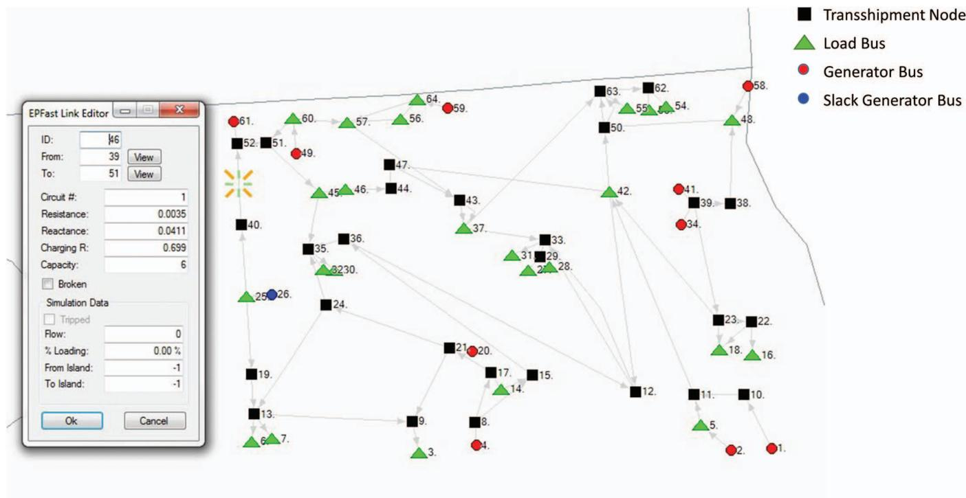
Fig. 2. (Color) *EPfast* depiction of a 64-bus network and associated link data
