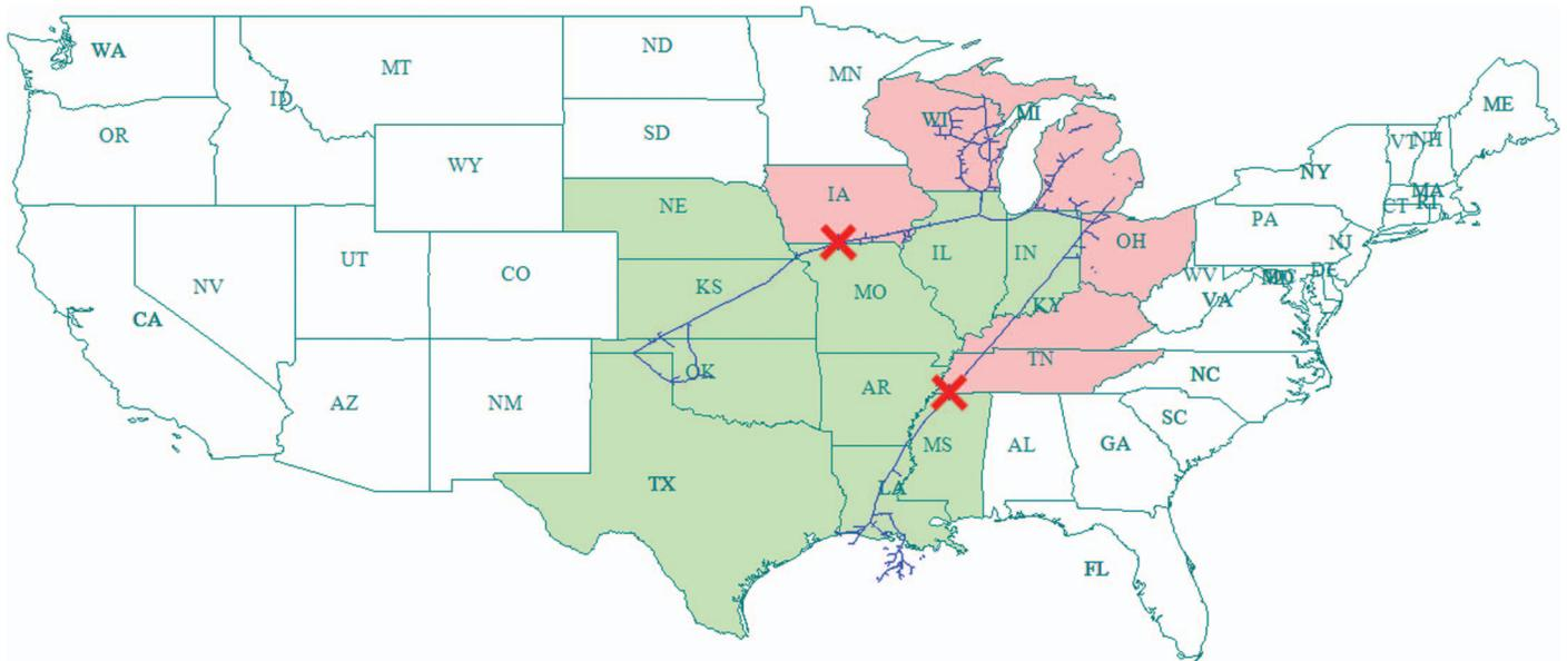
**Fig. 6.** (Color) *NGfast* graphical output for two notional pipeline breaks
