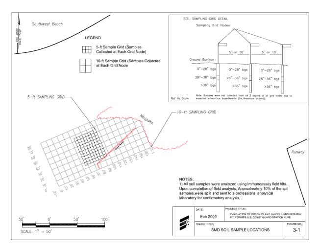
Figure C.1-4. Ten-foot and five-foot sampling grids used in 2008 ISM study. Source: USCG 2009, Figure 3-1.
