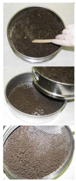
Figure 6-2. Example of wet-sieving soil on an as-received basis.
