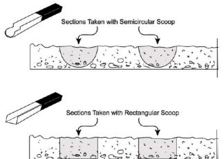
Figure 2-12. Illustration of the effects of sampling device design on particle sizes in a sample. *Source*: Gerlach and Nocerino 2003.
