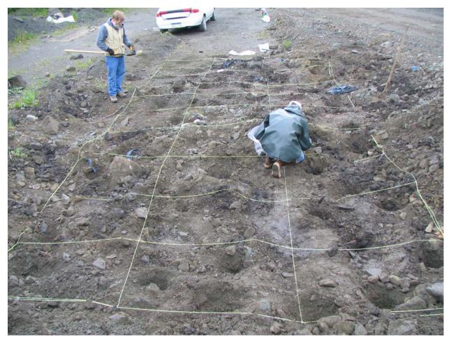
Figure C.2-4. Photograph showing increment collection.
