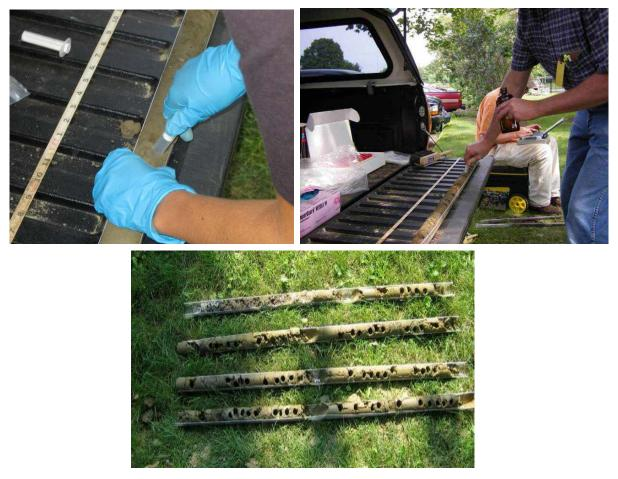
Figure 5-13. Example of sample increments being collected and added to a bottle containing methanol for preserving VOC samples.
