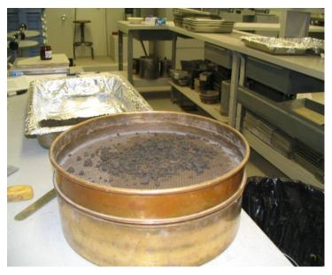
Figure C.2-5. Photograph of soil sifted through a #10 sieve.
