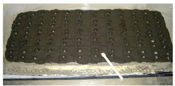
Figure 6-4. Example of 2-D Japanese slabcake incremental subsampling on moist sieved, "as-received" soil.
