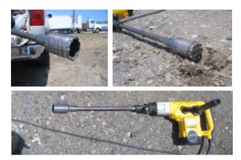
Figure 5-2b. Example of a drill core bit sampling tool for nonvolatile soil increment collection.
