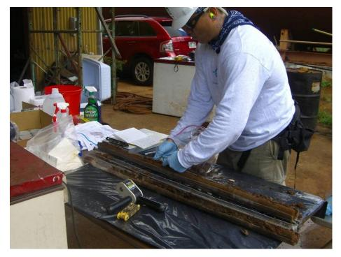
Figure 5-7. Example of removing a wedge from the entire length of a soil core.
