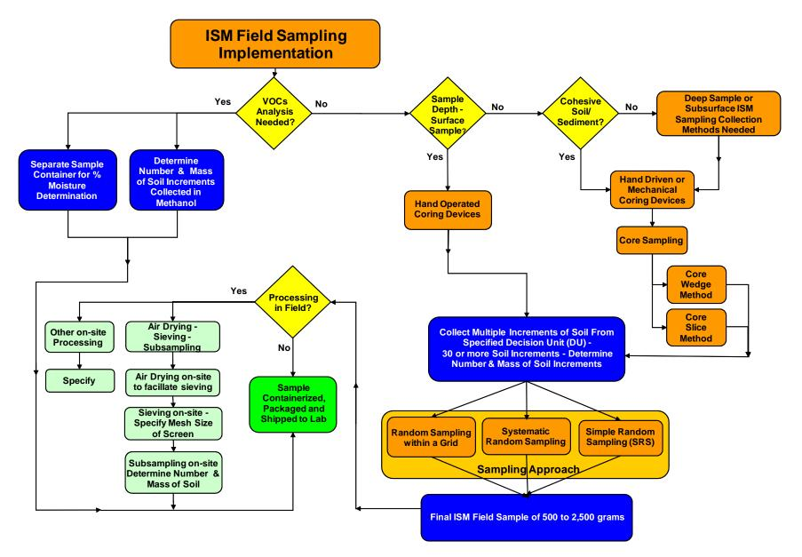
Figure 5-1. Field sampling implementation flowchart.
