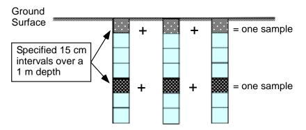
Figure 5-6. Schematic of a procedure to collect an ISM profile sample where two depths have been selected.
