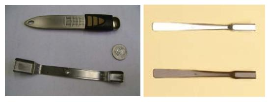
Figure 5-9. Examples of rectangular and flat-bottom sampling tools.
