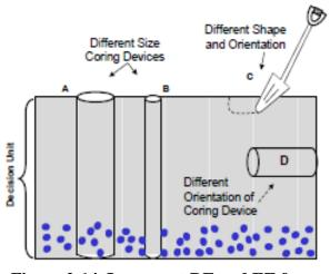
Figure 2-14. Increment DE and EE from sampling device selection. Source: USEPA 2002e.
