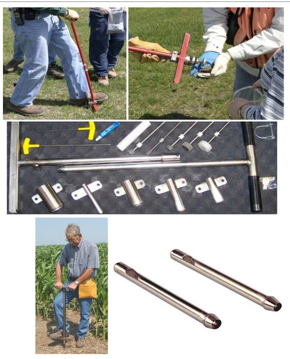
**Figure 5-2a. Examples of coring devices for nonvolatile soil increment collection.** Top to bottom: Multi-Incremental Sampling Tool (MIST<sup>TM</sup>), EVC Incremental Sampler, JMC Backsaver Handle, and Soil Tube.
