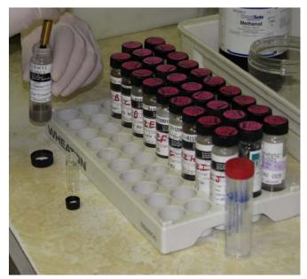
Figure 5-14. Example of methanol aliquots from individual 5 g field-preserved increments being combined in the laboratory.
