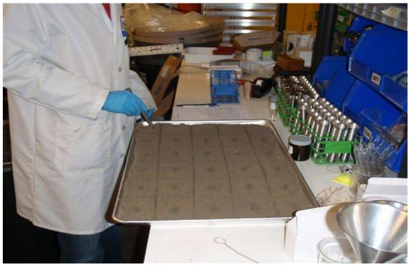
Figure 6-3. Example of 2-D Japanese slabcake incremental subsampling on dried and sieved soil.
