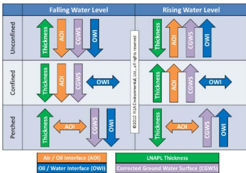
**Unconfined LNAPL:** During unconfined LNAPL conditions, all three interfaces and the LNAPL thickness will typically fluctuate. The apparent LNAPL thickness will fluctuate in the opposite direction of the three interfaces.
