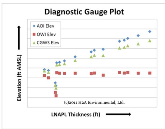
**TREND ANALYSIS:** Fluctuating AOI, OWI and CGWS elevations in equilibrium will exhibit diagnostic trends when plotted against the associated apparent LNAPL thicknesses gauged in the well. These trends can be used to screen for periods of unconfined, confined or perched LNAPL conditions.
