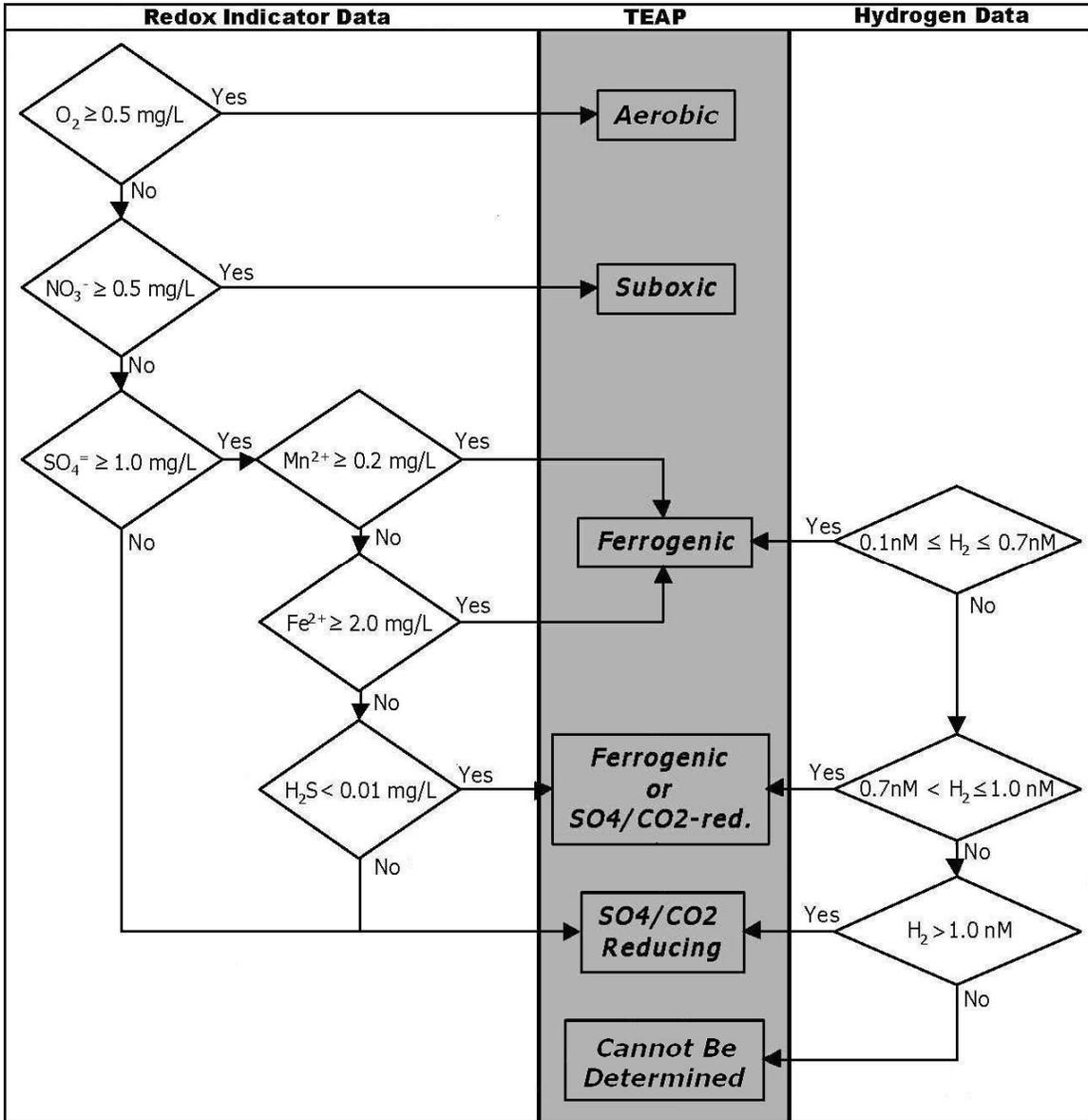
Figure 38. Flow Chart for Determining Redox Conditions
