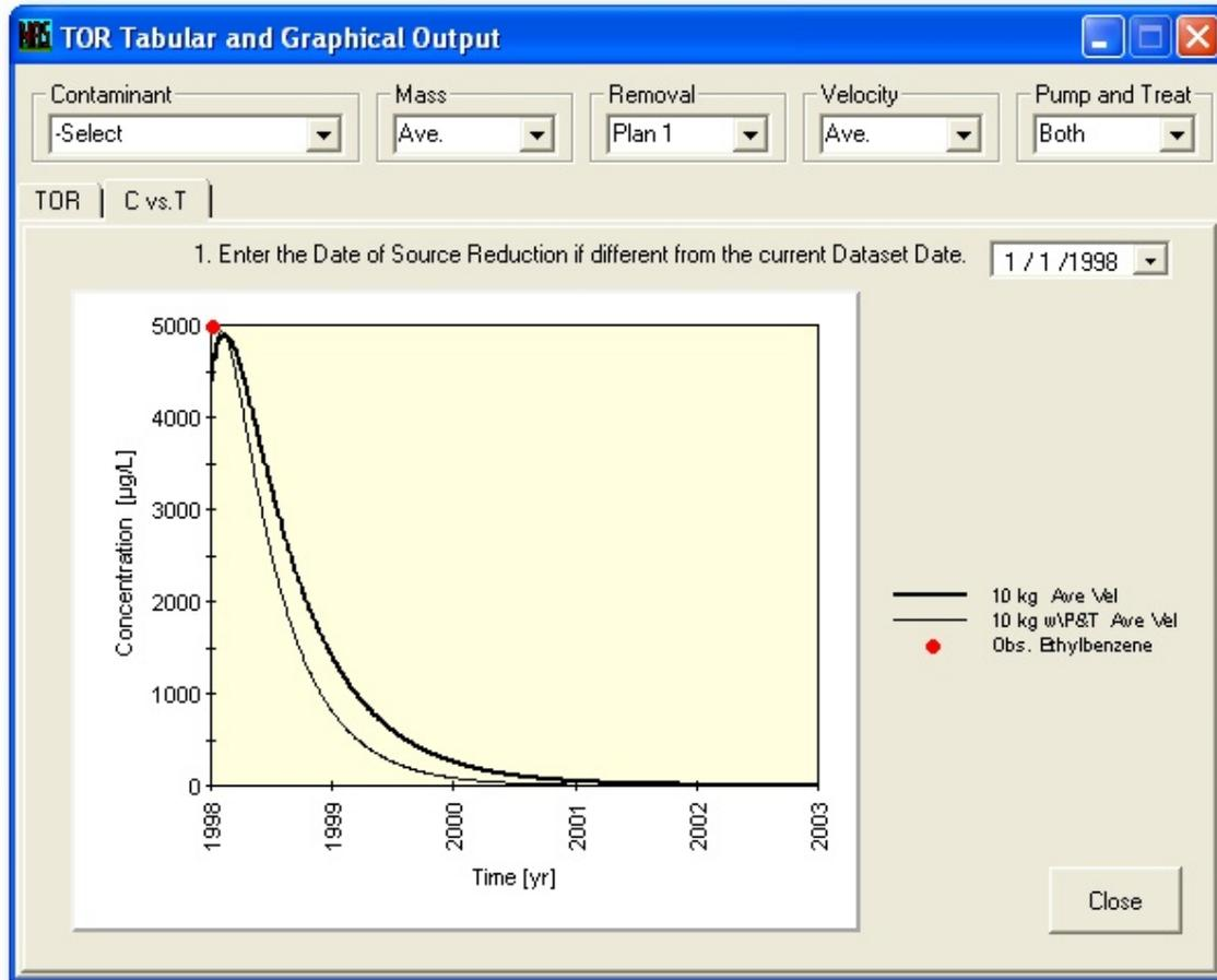
Figure 27. TOR – Graphical Output – Concentration vs. Time
