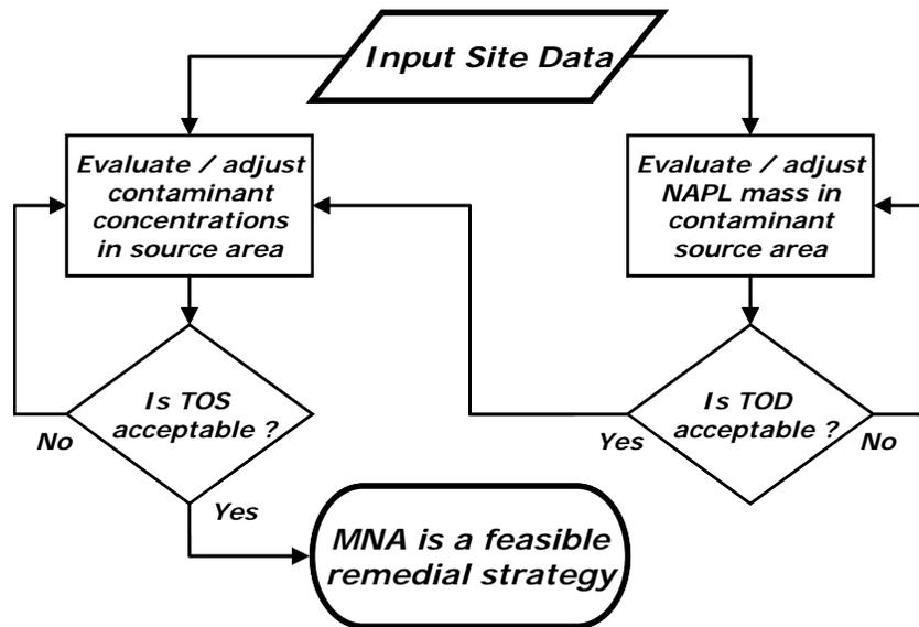
Figure 1. Flow Chart for the Application of NAS
