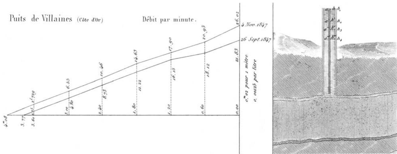
Figure 4. Spring flow measurements. Detail from Darcy [1856, Plate 22].
