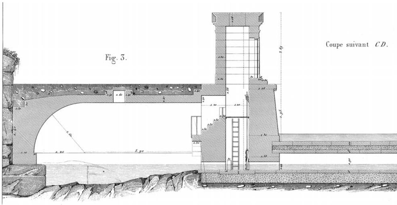
**Figure 2.** Section of Rosoir Spring Inlet Structure, covered aqueduct on the right. Detail from *Darcy* [1856, Plate 3].
