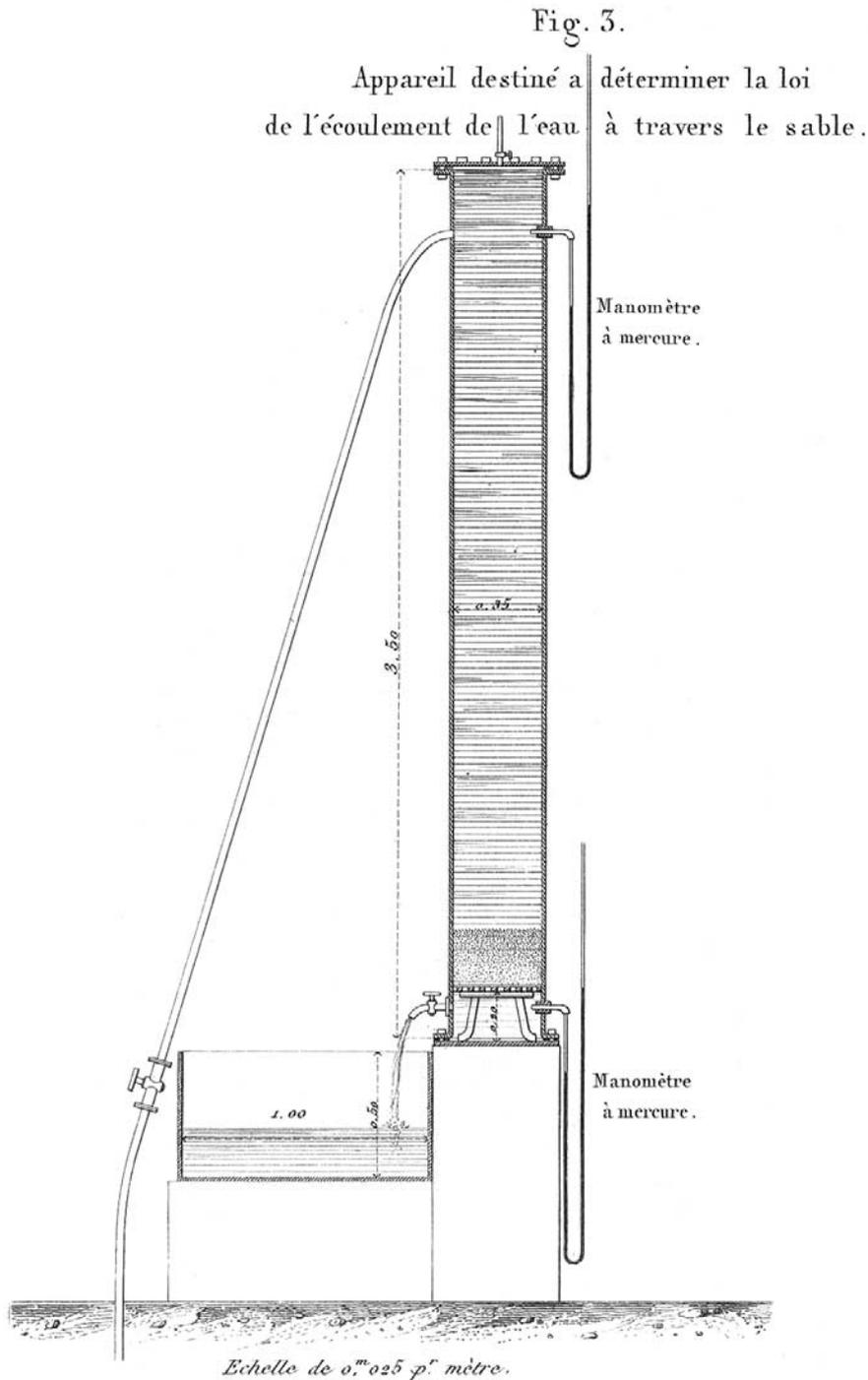
**Figure 5.** Column apparatus [Darcy, 1856, Figure 3, Plate 24].
