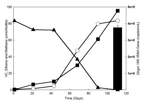
**Figure 4.3** VC degradation by culture GP (Fill triangle-VC; open circle-ethene; filled square-methane; filled bar- *Dhgm* 16S rRNA gene copy number). Data points are average of duplicate cultures; the error bars are one standard deviation, which are masked by the data symbols.
