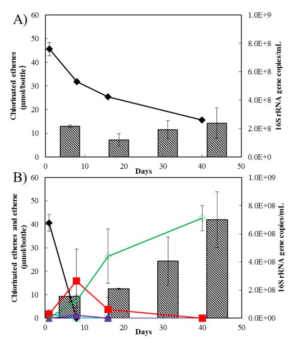
**Figure 3.1** PCE dechlorination at pH 5.5 and 7.2 by a PCE-to-ethene consortium containing *Dhc*. No dechlorination activity and growth of *Dhc* at pH 5.5; while PCE could be degraded to ethene at pH 7.2 coupled with *Dhc* growth. PCE loss at pH 5.5 was mainly due to abiotic loss (e.g. absorption to the stoppers). (Filled black diamond-PCE, empty blue square-TCE, filled purple triangle-*c*DCE, filled red square-VC, empty green diamond-ethene, shaded bar-*Dhc* 16S rRNA gene copy number).
