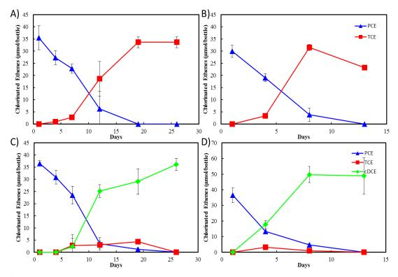
**Figure 2.3** *Sulfurospirillum* isolates strain PLC-TCE and PLC-DCE, which dechlorinate PCE to TCE (A-pH 5.5; B-pH 7.2) and *c*DCE at pH 5.5 (C-pH 5.5; D-pH 7.2), respectively. The isolates were cultivated with lactate and hydrogen as carbon source and electron donor. Error bars represent one standard deviation below or above the average of duplicate samples. (Blue Triangle-PCE, Red Square-TCE and Green Diamond-cDCE).
