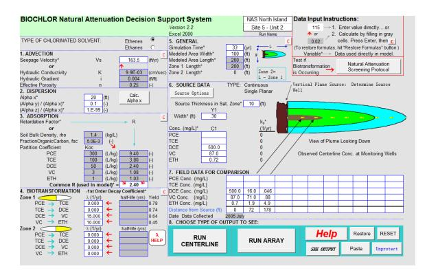
Figure 5.1 Input screen of Biochlor. NAS North Island Site 5 Unite 2, CA.
