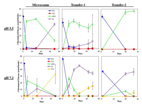
**Figure 2.1** PCE dechlorination by microcosms and transfer enrichments of ACS sample under different pH conditions (First row-pH 5.5, demonstrating PCE could be degraded to VC under microcosm condition, but only PCE-to-cDCE dechlorination could be repeatedly transferred; Second row-pH 7.2, demonstrating PCE-to-ethene dechlorination could be maintained). All figures show the results from average of triplicate serum bottles.
