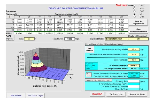
Figure 5.3 Array concentration output for VC. NAS North Island Site 5 Unite 2, CA. 130
