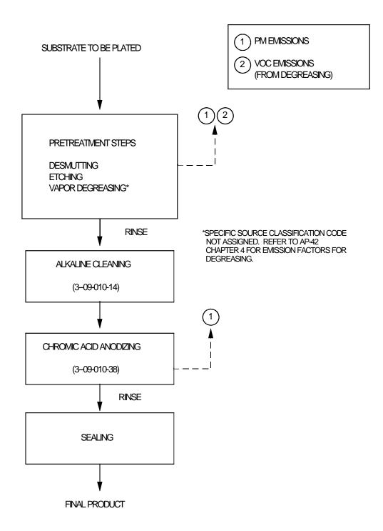
Figure 2-3. Flow diagram for a typical chromic acid anodizing process.<sup>3</sup> (Source Classification Codes in parentheses).
