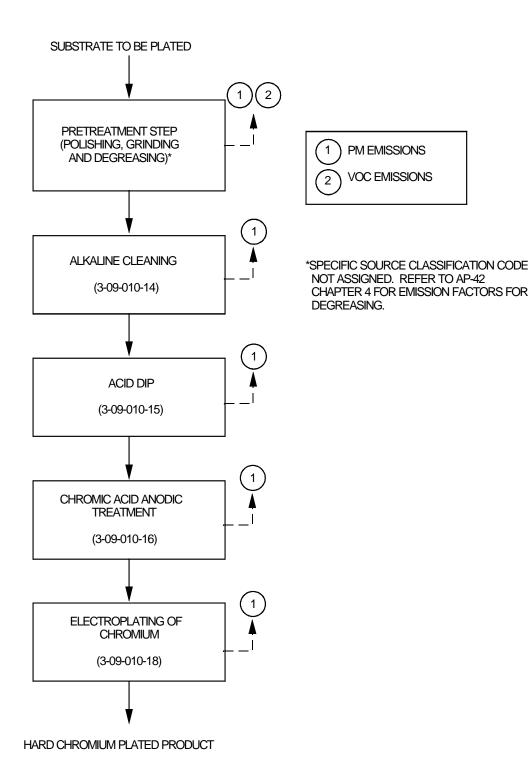
Figure 2-1. Flow diagram for a typical hard chromium plating process.<sup>3</sup> (Source Classification Codes in parentheses)
