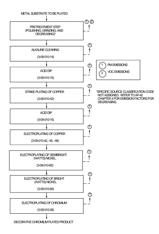
Figure 2-2. Flow diagram for decorative chromium plating on a metal substrate.<sup>3</sup> (Source Classification Codes in parentheses).
