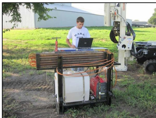
dissipation tests are performed down-hole. The field instrument receives signal input from the string pot (depth encoder), flow controller, pressure sensor and Wenner array. That data is transferred in digital format from the field instrument to the operator's computer.
