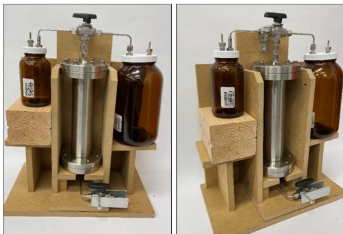
Figure 4-9. Prototype column apparatus for Draft Method 1314A: front and side views showing eluate collection in 250-mL and 1250-mL amber glass bottles.
