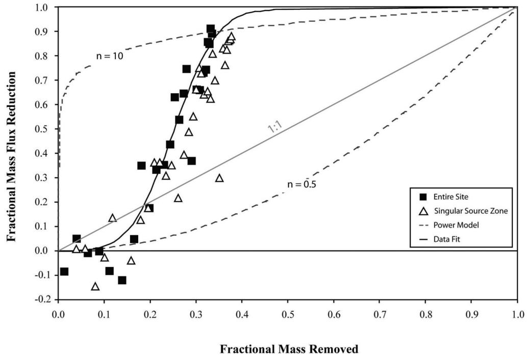
**Figure 6b.** Mass-flux-reduction/mass-removal relationship for the entire TIAA site excluding the initial aqueous-phase mass associated with the plume; and comparison to the mass-flux-reduction/mass-removal relationship for one specific source zone. The dashed lines represent curve simulated using the simple mass-removal function (Equation 3). The solid line was fit to the data using a cumulative distribution function.
