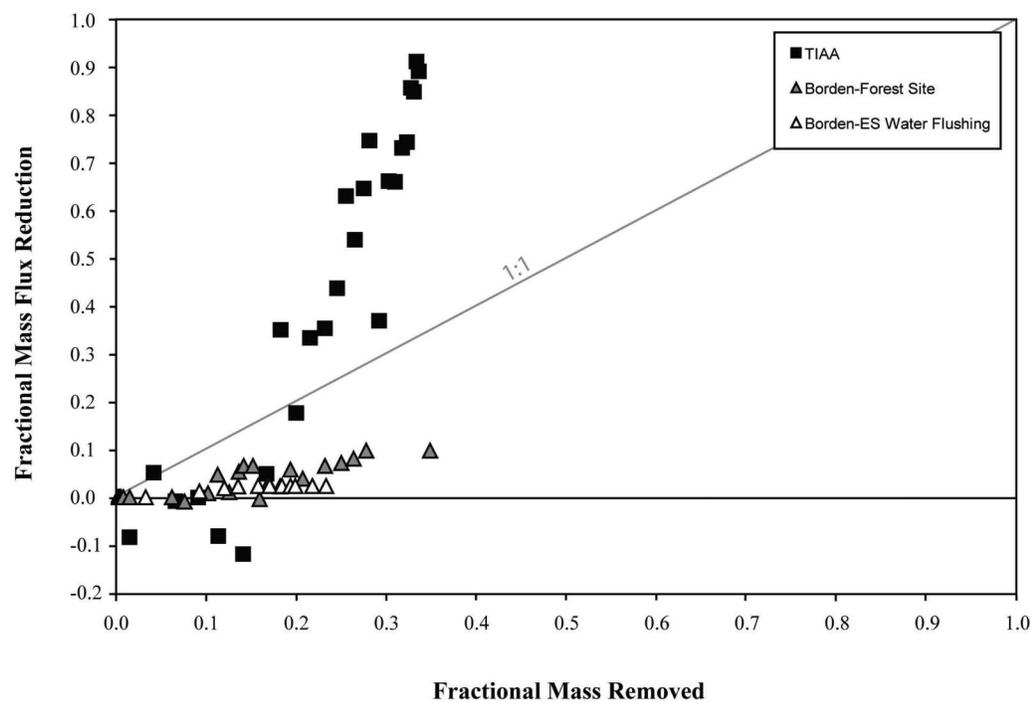
**Figure 7.** Comparison of the mass-flux-reduction/mass-removal relationships for three aqueous flushing field studies.
