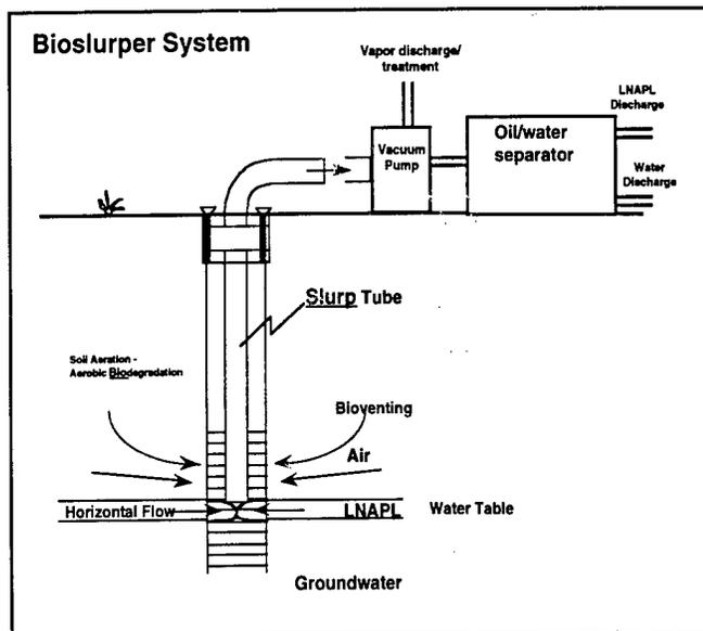
Bioslurping is an approach adapted from the vacuum dewatering industry. A bioslurper system consists of a "slurp" tube that extends into the LNAPL free product layer in the well. Product is drawn into the tube as air
